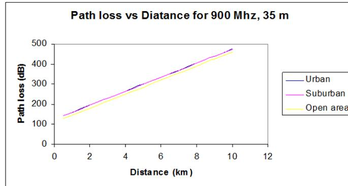
Figure 2: Path loss for 900 MHz, at 35 m base antenna height
