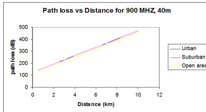
Figure 3: Path loss for 900 MHz, at 40 m base antenna height
