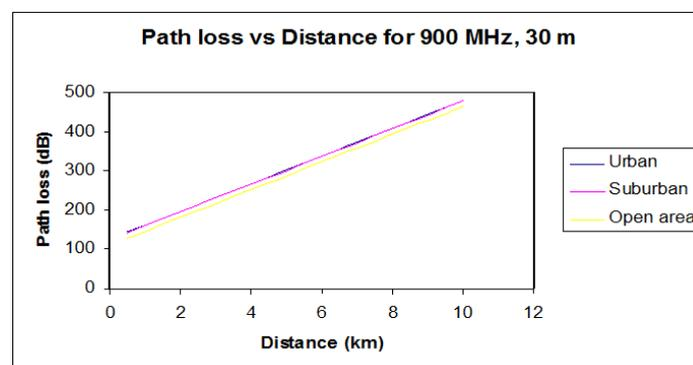
Figure 1: Path loss for 900 MHz, at 30 m base antenna height
