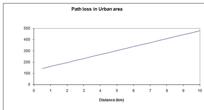
Figure 4: Path loss for 900 MHz, at 30 m base antenna height for Urban environment
