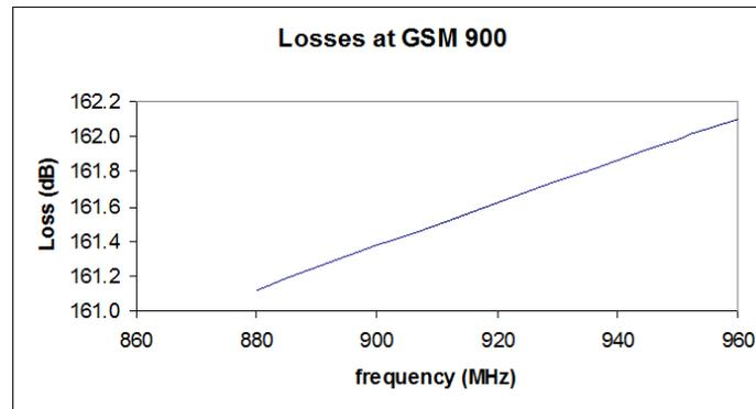
Figure 5: Path loss for GSM 900 at 30 m base antenna height for Urban environment
