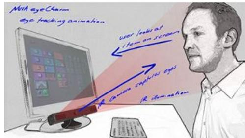
**Figure 1:** *Process of Tracking*
