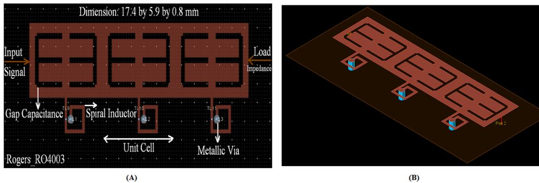
**Figure 2:** Configuration of the proposed concise UWB MTM antenna composed of the three unit cells based on CRLH-TL. A) Top view, B) Isometric view.
