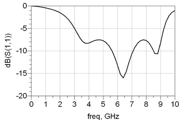
Figure 3: Simulated return loss ( $S_{11}$ ) parameter.
