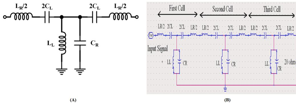
**Figure 1:** Equivalent circuit model of the proposed Antenna based on CRLH MTM-TL for: A) One unit cell, B) Entire structure.
