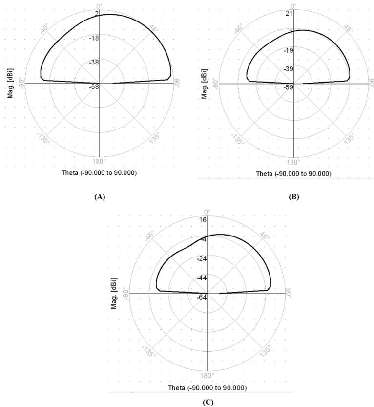
**Figure 4:** The Radiation Patterns (Gains) of the proposed antenna in elevation ( $\phi=0$  degree), A) 5.6 GHz, B) 6.4 GHz and C) 7.1 GHz.
