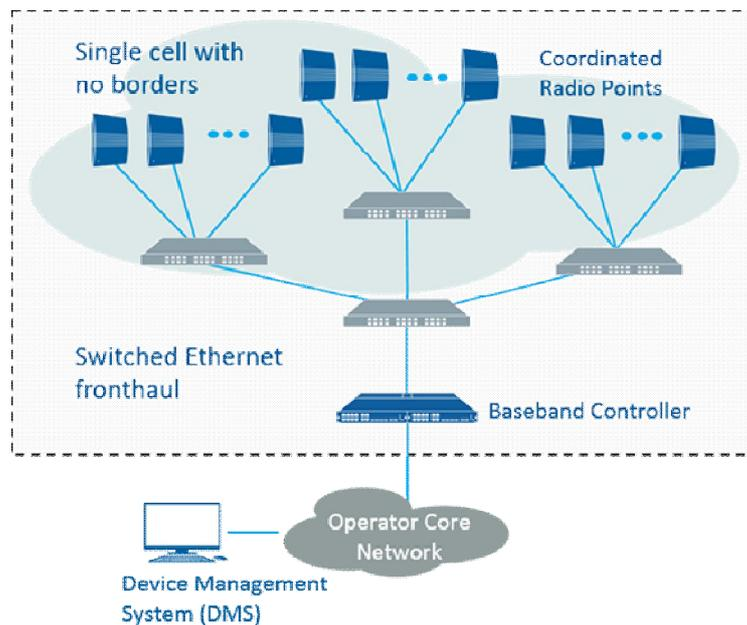
Fig. 4: In OneCell's C-RAN architecture, baseband processing is centralized in the Baseband Controller to create a single cell without border interference or handovers [Source: Wikipedia]
