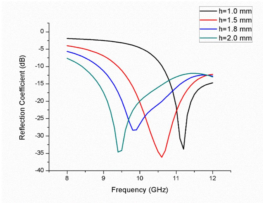
Figure2: Variation of bandwidth with different height of substrate.
