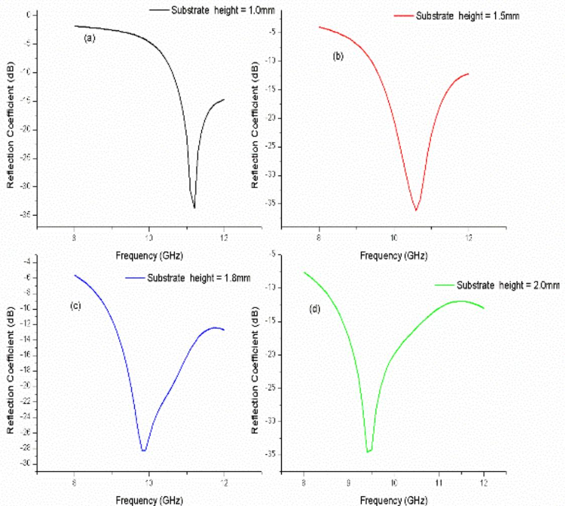
Figure 1: Set of variation in bandwidth with variation in the height of Substrate.
