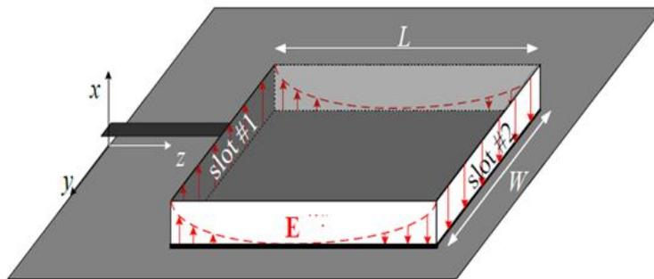
Figure 8: Electrical field Distribution in Microstrip Antenna using Transmission Line Model
