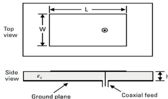
Figure 3: Microstrip Antenna fed by Coaxial Probe Feed
