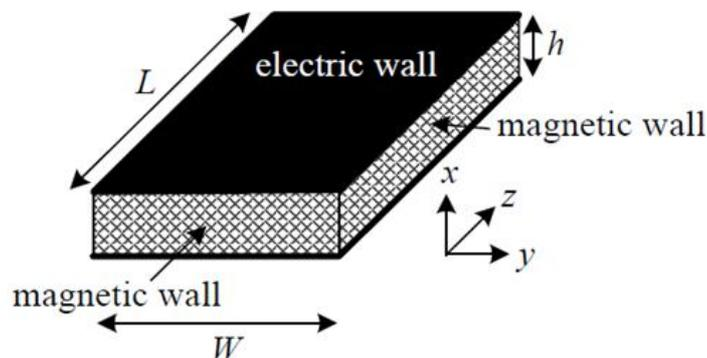
Figure 9: Representation of Microstrip Antenna using Cavity Model
