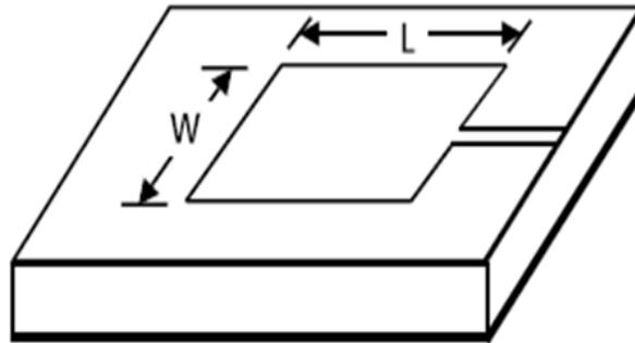
Figure 2: Microstrip Antenna fed by Microstrip Line Feed
