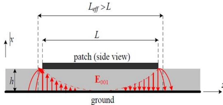
Figure 7: Representation of Microstrip Antenna using Transmission Line Model
