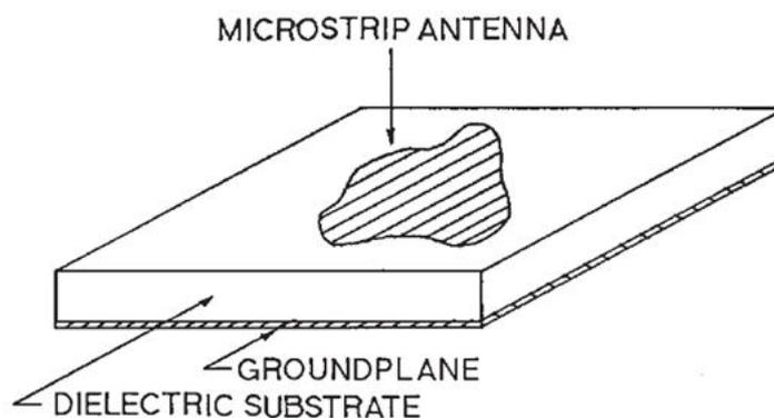
*Figure 1: Geometry of a Microstrip Antenna*
