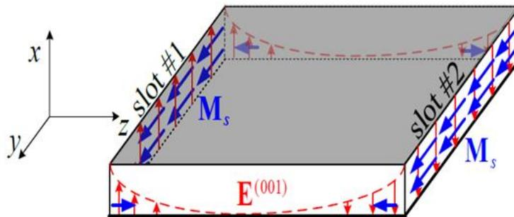
Figure 10: Magnetic Field Distribution in Microstrip Antenna using Cavity Model
