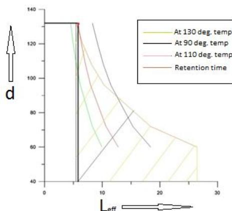
Figure 3:  $d$  and  $L_{eff}$  at different temperatures
