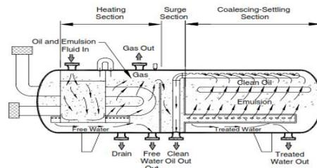
Fig. 2: Horizontal heater treater
