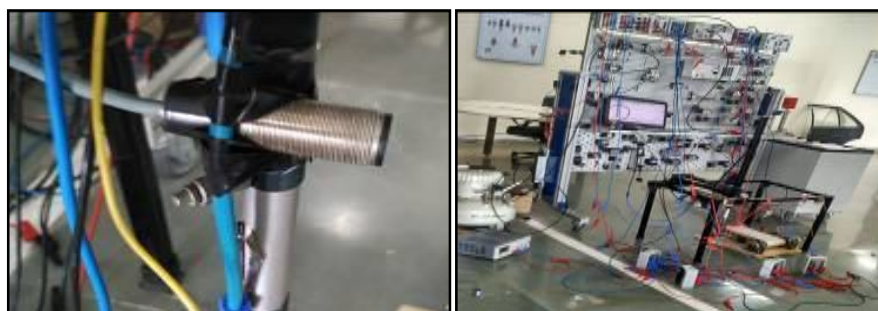
Figure 4: Proximity sensor for obstacle detection and PLC-robot interfacing
