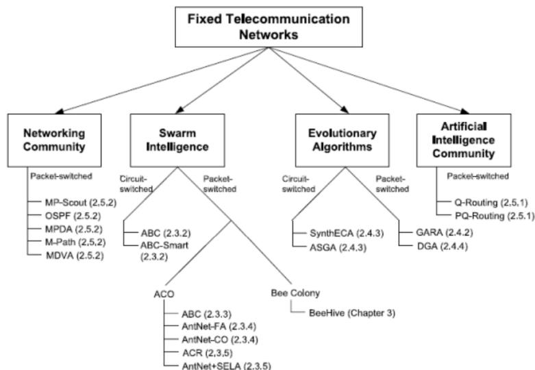
Figure 1: Routing protocols for telecom networks
