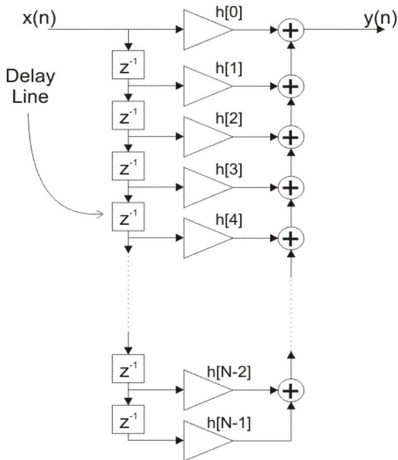
Figure 3: Direct form of FIR filter realization
