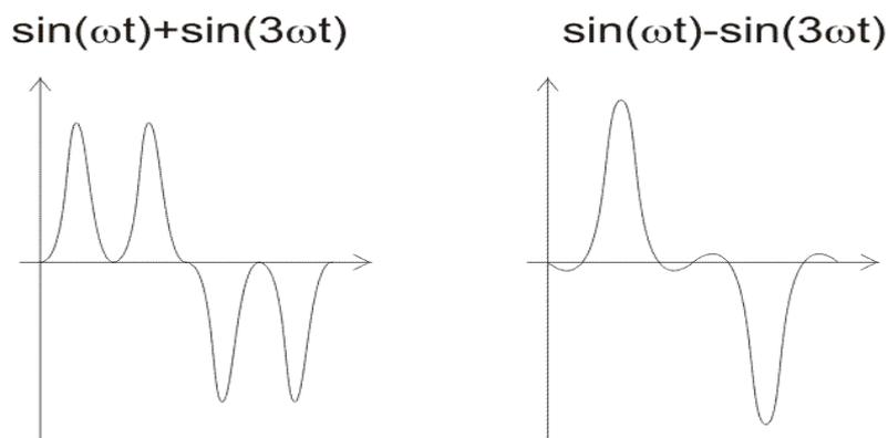
Figure 2 The effect of non-linear phase characteristic
