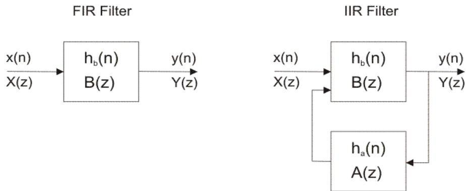
Figure 1: FIR and IIR filters block diagram
