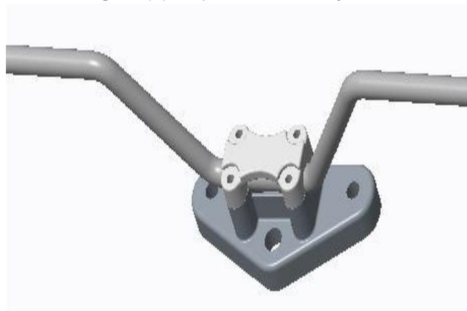
Figure (2): New designed triple tree.
