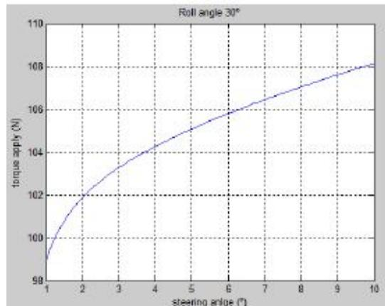
Figure (5): Steering angle vs. steering torque at roll angle 30°
