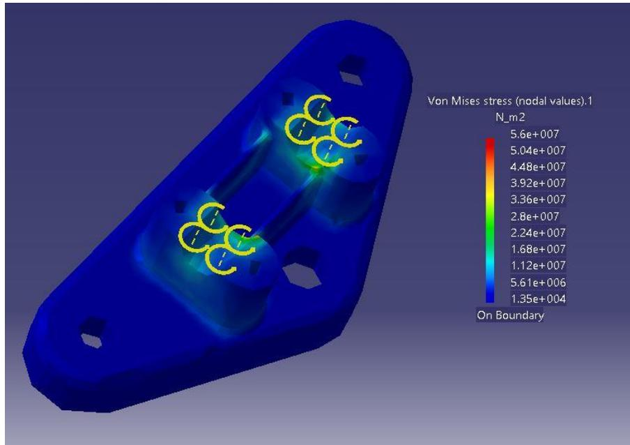
Figure (8): Von Mises stress on application of steering torque.
