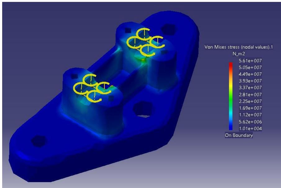
Figure (10): Von Mises stress on application of combined steering torque and force.
