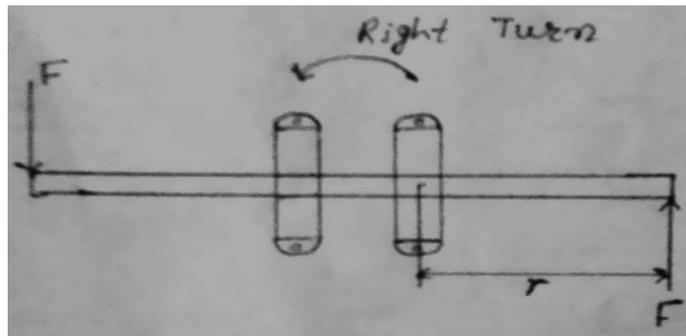
Figure (4): Steering torque on handlebar
