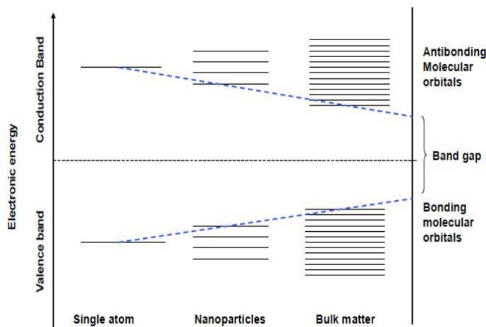
Fig.4: Diagram of band gap change in Nanoparticles
