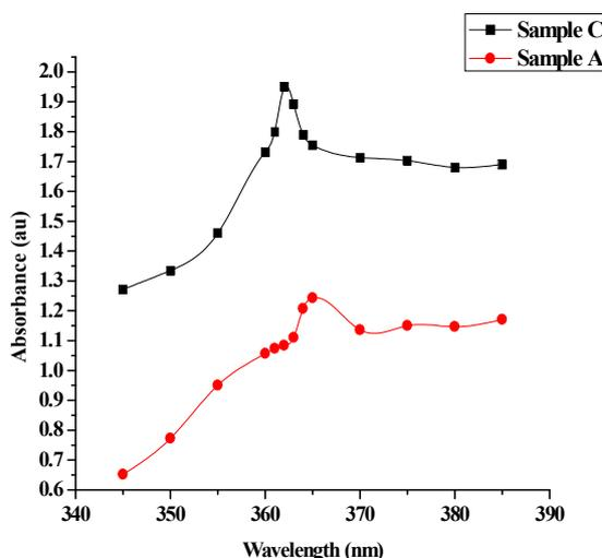
Fig. 2: UV of ZnO Nanoparticles prepared by 0.5ml (upper) and 0.12ml (lower) thioglycerol
