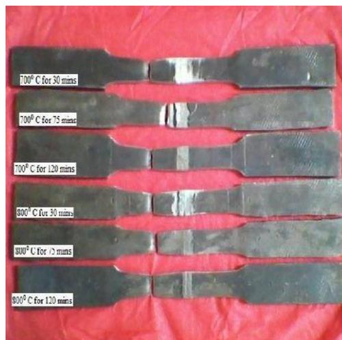
Figure 4: Specimens after sensitization and tensile test.
