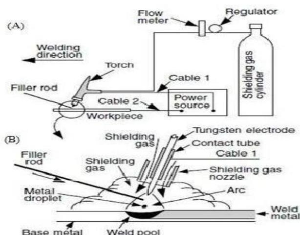
Figure 2: GTAW: (A) overall process, (B) welding area enlarged. [28]
