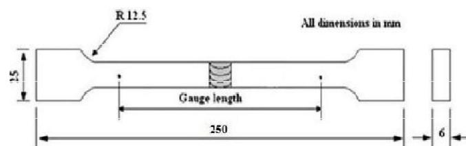
Figure 3: Tensile specimen.
