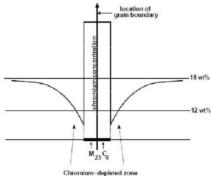
Figure 1: Grain boundary microstructure in sensitized austenitic stainless steel. [7]
