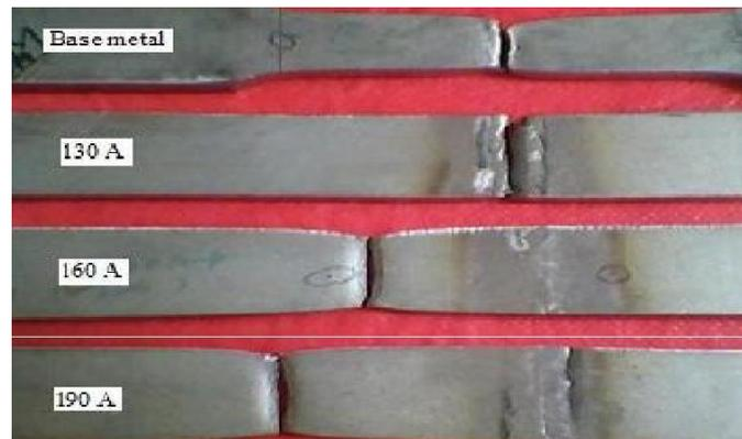
Figure 4.. Specimens after welding and tensile test.
