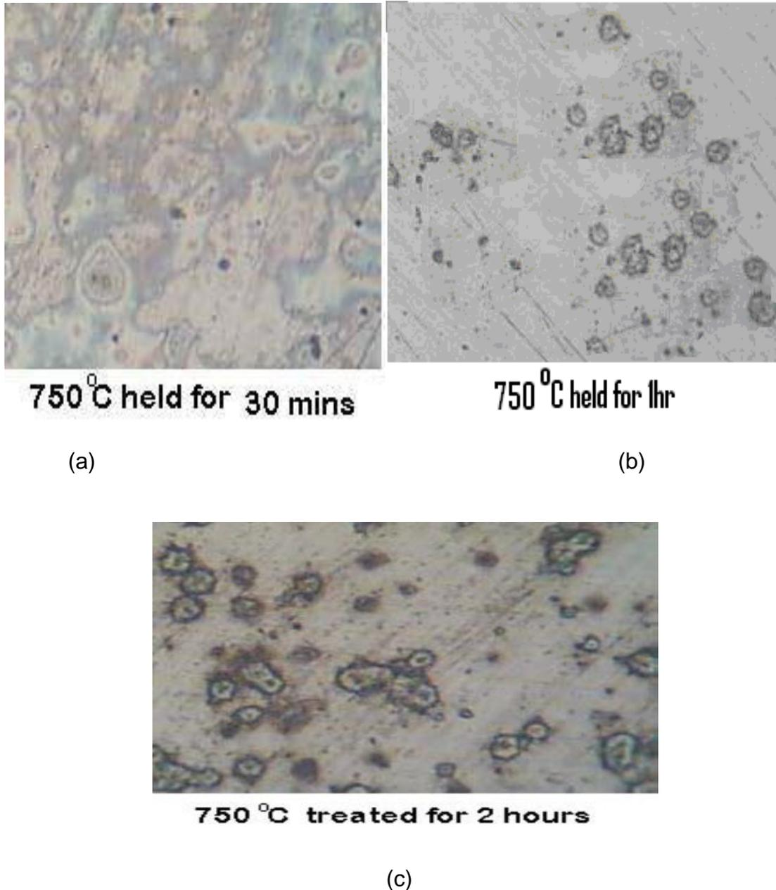
*Figures 5. (a) Sample heated to 750 °C held for 30mins, (b) Sample heated to 750 °C held for 1hr, (c) Sample heated to 750 °C held for 2hrs*
