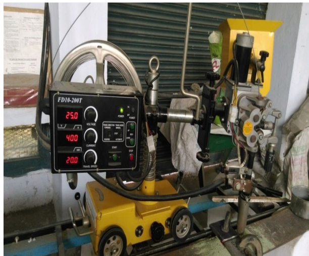
Figure 1:-setup of submerged arc welding
