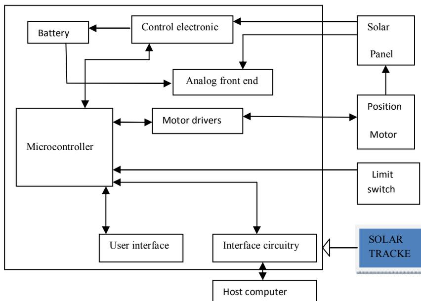
*Fig.2 block diagram of solar tracker system*
