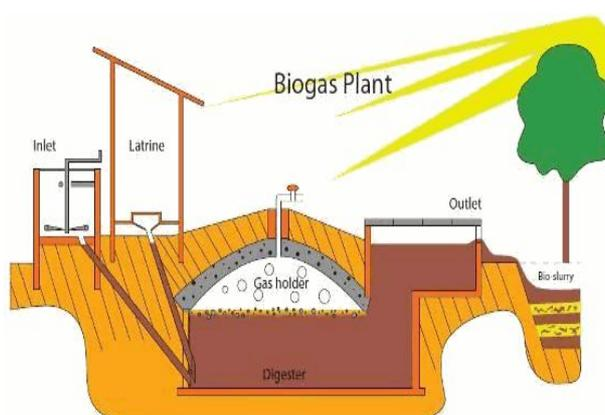
Figure 1: Components of Biogas Plant
