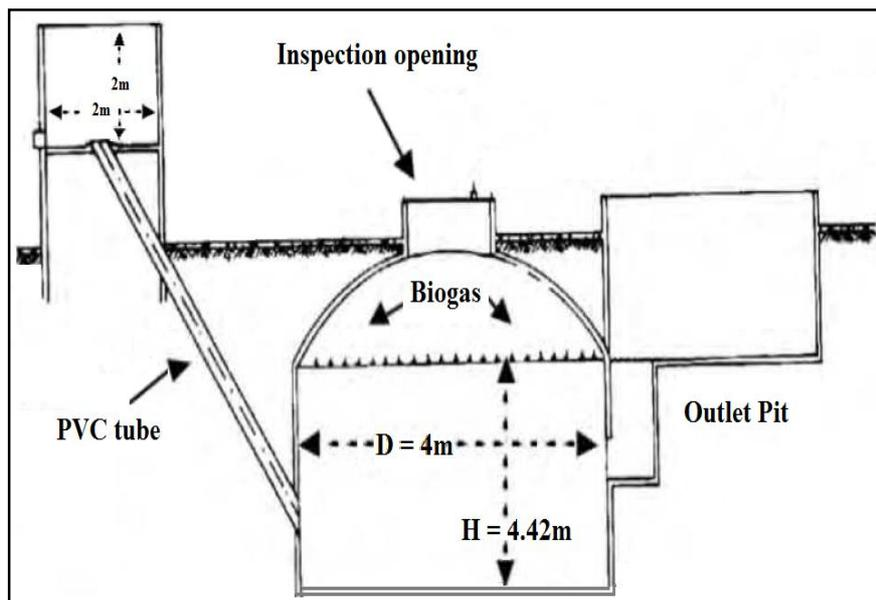
Figure 2: Propound Design of Biogas plant at LDRP – ITR, Gandhinagar
