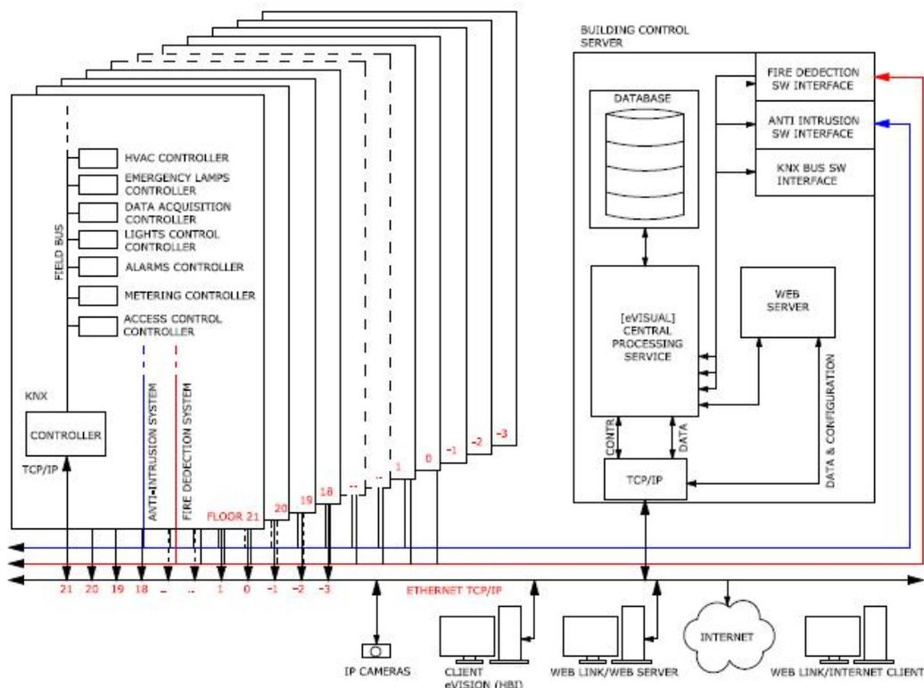
Figure 2 - A typical architecture of the automation system used in buildings of figure 1
